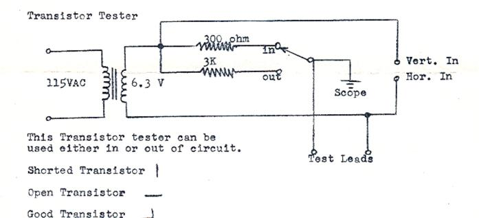
To check in circuit put switch in position indicated.
